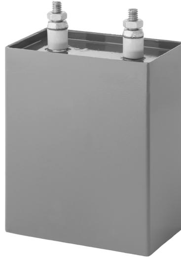
Pulse forming networks are designed for use in circuits which convert direct current or sinusoidal alternating current to unidirectional square pulses at high energy levels for short duration. The performance of the pulse forming network is the heart of the modulator for radar or missile operation.
