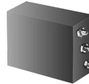
Hermetically sealed, oil filled, rectangular phenolic tube. The illustration shows the means of enclosing three .03 mfd 10 KV capacitors in one case. One stud (not seen) is common to all of three capacitors. Size is 1 1/4"x 2"x 2 3/4"
